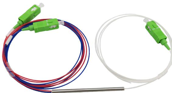
Single mode Coupler 1x2, 2x2 offer very low insertion loss, low polarization dependence and excellent environmental stability. Accurate coupling ratio from 50/50 to 1/99, fiber type 250um bare fiber, 3mm and 900um loose tube fiber are available with very tight uniformity in a wide wavelength. It is applicable to perform power splitting and monitoring functions in all kinds of optical communication systems.
