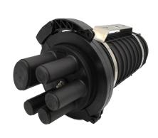
FOSC400A4 fiber optic splice closures are specially designed to protect joints of optic cable. Excessive fibers can be stored in storage baskets behind the splice trays. The optical fibers are fusion on sides of the tray. One tray can splice 24 fibers; Available for 6 trays to splice total 144 fibers. Adopt modified PP material, with anti-UV, anti-aging and corrosion resistance material. Good quality and long service life. It is reusable.
